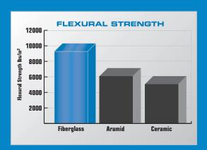
Abex® linings' high fiberglass content gives them superior flexural strength. Fiberglass has 50% more flexural strength than other brake lining fibers.
