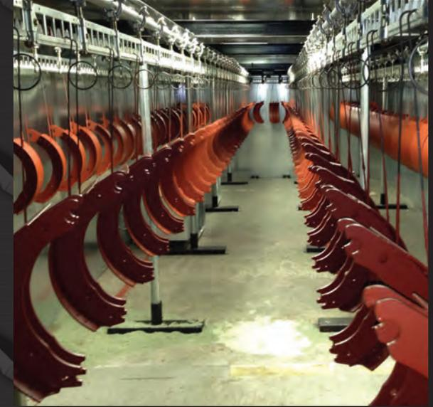
The BMS Fully Automatic Prep - Paint - Dry Process provides consistently clean brake shoes in only a fraction of the time from start to finish meaning a better looking and longer lasting product that ECRB can confidently sell to their customers.
