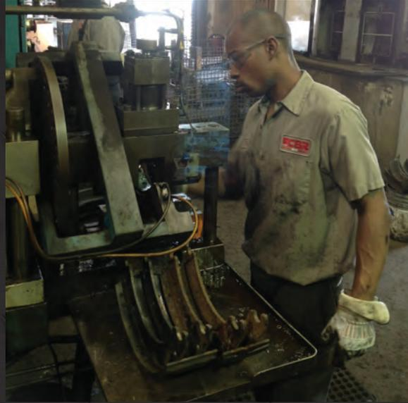
The worn down lining must be removed from the shoe. The lining is held on to the steel brake shoe with locked steel rivets. The rivets are removed with BMS Auto Deliners by punching through the rolled down clinch of the rivet and then push the rivet body out of the table of the brake shoe and lining without causing table damage that often occurs with other de-lining methods.
