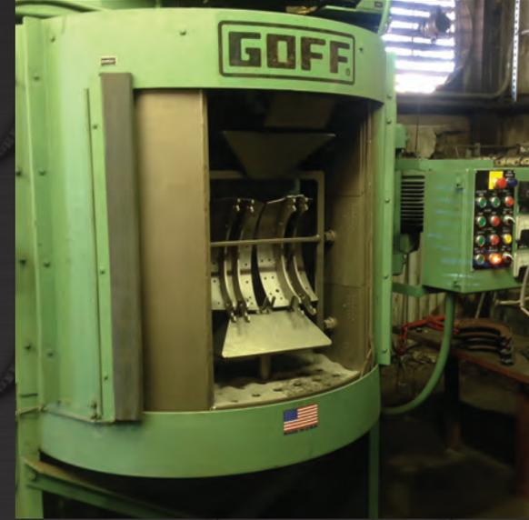
The steel brake shoe is shot blasted with millions of steel balls moving at 150mph to remove all paint, scale and rust so that the brake shoe is down to bare steel and has proper surface for paint to adhere.
