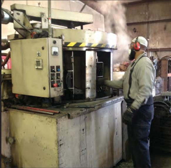
Each brake shoe is washed with water at 50psi at 195°F with large nozzles that remove all of the oil & grease with a BMS Washing Machine, the industry standard. The brake shoe is then visibly clean, hot & ready for removing the lining.
