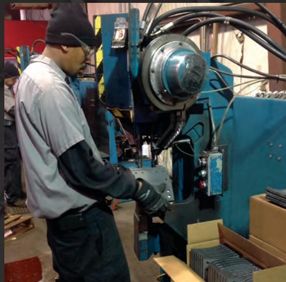
Finally, BMS hydraulic riveters are used to install the new brake lining to the brake shoe. These hydraulic machines compensate for variances in the thickness of the brake shoes, lining & rivets and eliminates any loose lining. Premium steel rivets are used which give the most secure & reliable fastening solution in the truck brake industry. The rivets completely remove all rivet collapse and tube split in the process, which means higher quality for our customers.
