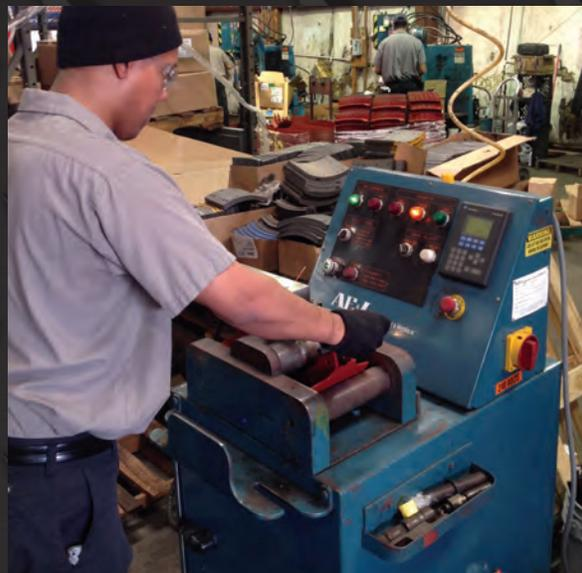
All brake shoes are checked for stretch, compression, anchor pin and cam roller looseness. These brake shoes will be brought back to OEM specifications (with the exception of compressed shoes) with our EATON Brake Shoe Straightening Machine. During the correction process the gauge monitors the span of the shoe to avoid over-bending.
